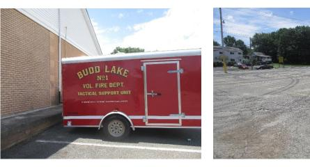
Parking spaces north and east of the building can be replaced with porous asphalt to infiltrate stormwater. Rainwater can be harvested by installing a cistern at the northeast corner of the building for washing trucks. A preliminary soil assessment suggests that the soils have suitable drainage characteristics for green infrastructure.
