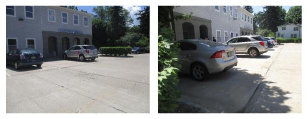
Parking spaces west of the building can be replaced with porous asphalt to infiltrate stormwater. A preliminary soil assessment suggests that the soils have suitable drainage characteristics for green infrastructure.
